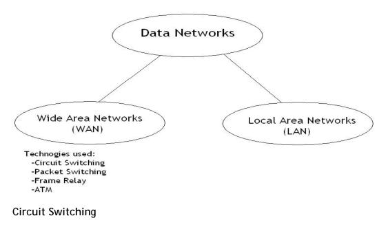
In a circuit-switched network, a dedicated communications path is established between two stations through the nodes of the network. That path is a connected sequence of physical links between nodes.
