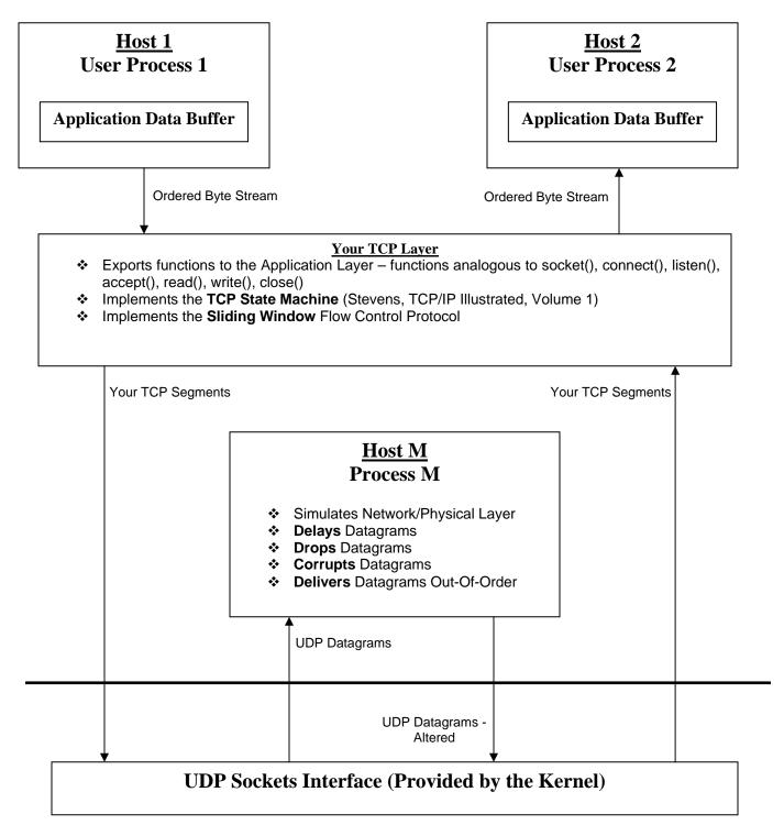
Since on a LAN, UDP is practically as reliable as TCP, we need another process M to simulate the Network Layer and Physical Layer. It introduces various anomalies in the UDP Datagrams. This process should be invisible to the actual communicating processes.
